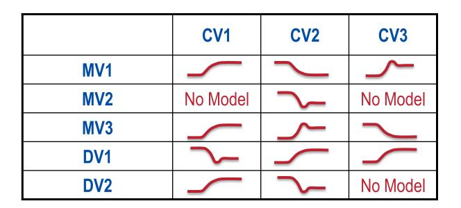
The completed MPC model will allow the controller to <u>PREDICT</u> the values of the CVs by movement of all the MVs and DVs. Hence <u>PROACTIVE</u> control can be taken to achieve the CVs setpoint before the they are violated, hence reducing variability
