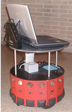
Fig. 1. Our mobile robots equipped with 3D sensors. Top image, Powerbot robot with laser Sick and a sweeping unit. Bottom, Magellan-Pro using a Digiclops stereo camera
