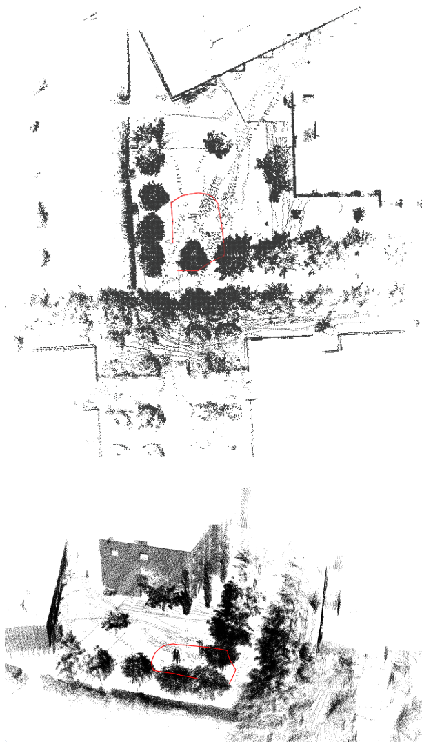
Fig. 8. First experiment results. Top image shows zenithal view of the complete map computed. Robot movement was obtained, from an outdoor semi-structured environment, using 6DoF planar patches based registration. Red line shows the registered trajectory obtained. Bottom, free 3D view of the first experiment computed map. We can observe some 3D objects like building walls, windows, trees, etc.
