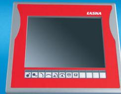
front mebrane design with modified colour scheme und different size mebrane keys
