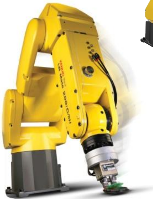
LR Mate 200iC/5H 5 ejes - 5 kg R = 704 mm
