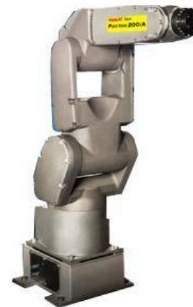
Paint Mate 200iA Paint Mate 200iA/5L 6 ejes - 5 kg R = 704 mm / 892 mm
