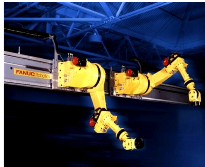
R-2000iB/200T 6 ejes – 200 kg R=2207mm
