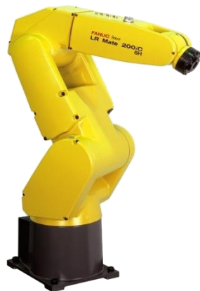
LR Mate 200iC/5H 5 ejes - 5 kg R = 704 mm
