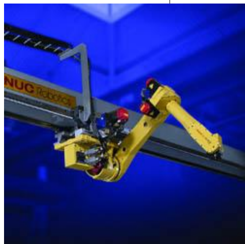
M-16iB/20T 6 ejes – 20 kg R=1513 mm
